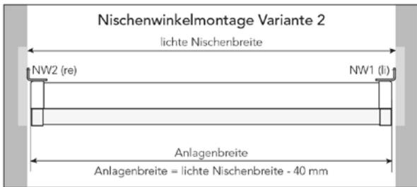
The system width can be determined as described on the previous page. (see page „Determining the system width“)
